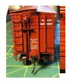
The door guides were then mounted and the long grab rails were put in position below the door openings. The doors were then mounted in the proper position.
